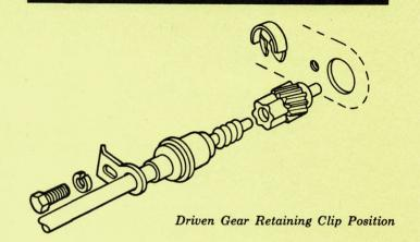
2. Whenever a drive gear is replaced, a new driven gear should also be installed.
