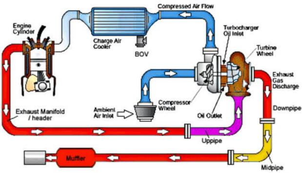
A turbocharger uses engine exhaust gasses to power a compressor that supplies combustion air to the engine. The increased supply of air allows more fuel to be introduced. The combination of more air and fuel produces more horsepower.
