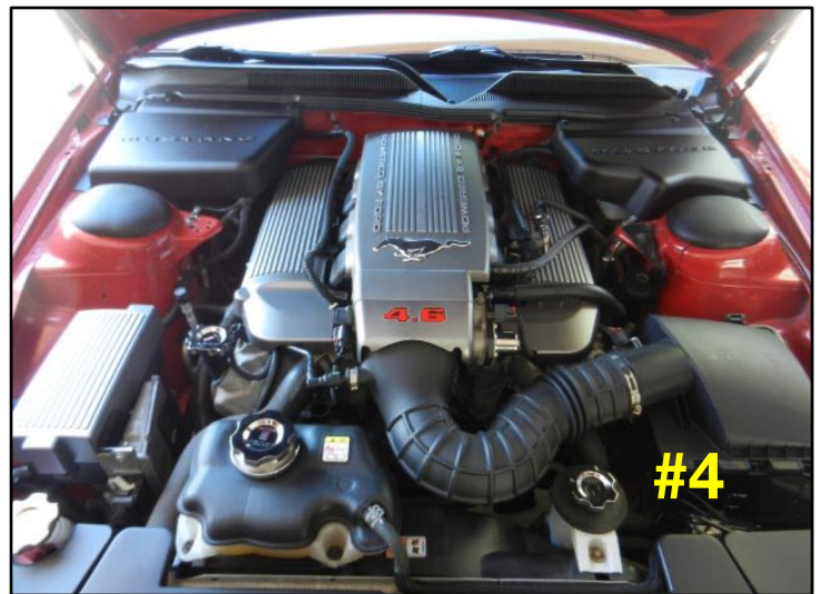
Engine has plenum & fuel rail covers. Sturt, battery & master cyl covers. chrome fluid caps.
