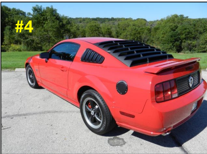
Rear window lovers, carbon fiber wrap gas filler, front fender hash stripes, trunk lid black out.
