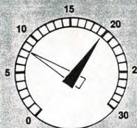
4. Leaking head gasket. Pointer will drop sharply at regular intervals when affected cylinder(s) try to fire.
