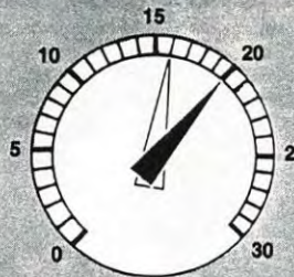
5. Leaking valves. Regular drop of 2-5 inches each time bad valve(s) try to close.
