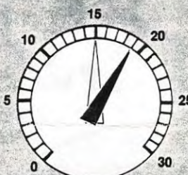
7. Sticking valve. An intermittent drop of 3-4 inches.
