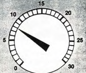
9. Late valve timing. A steady but very low reading at idle.
